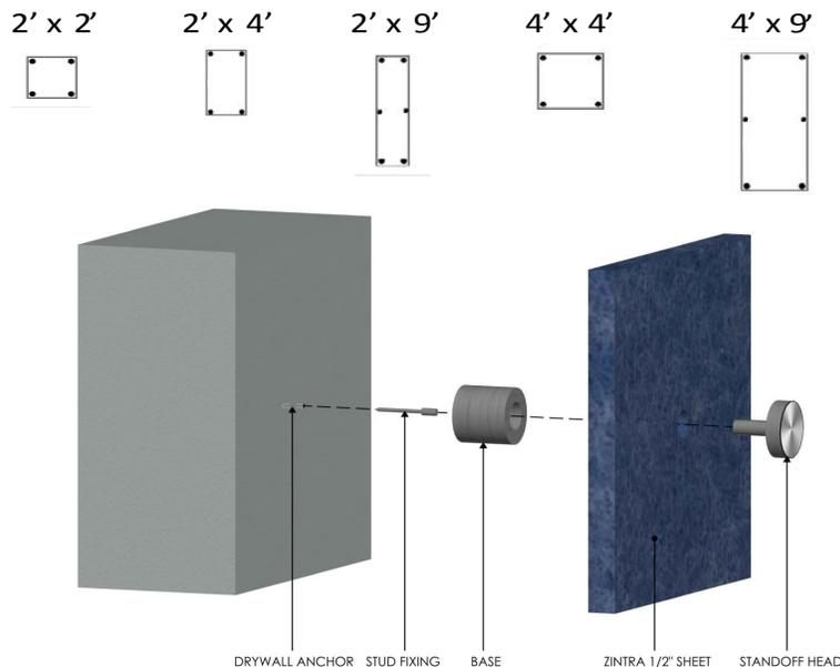
Begin by marking the panel back for the placement of each hole for each stand-off required. No hole should be closer than 3" away from the perimeter edges of the panel.
